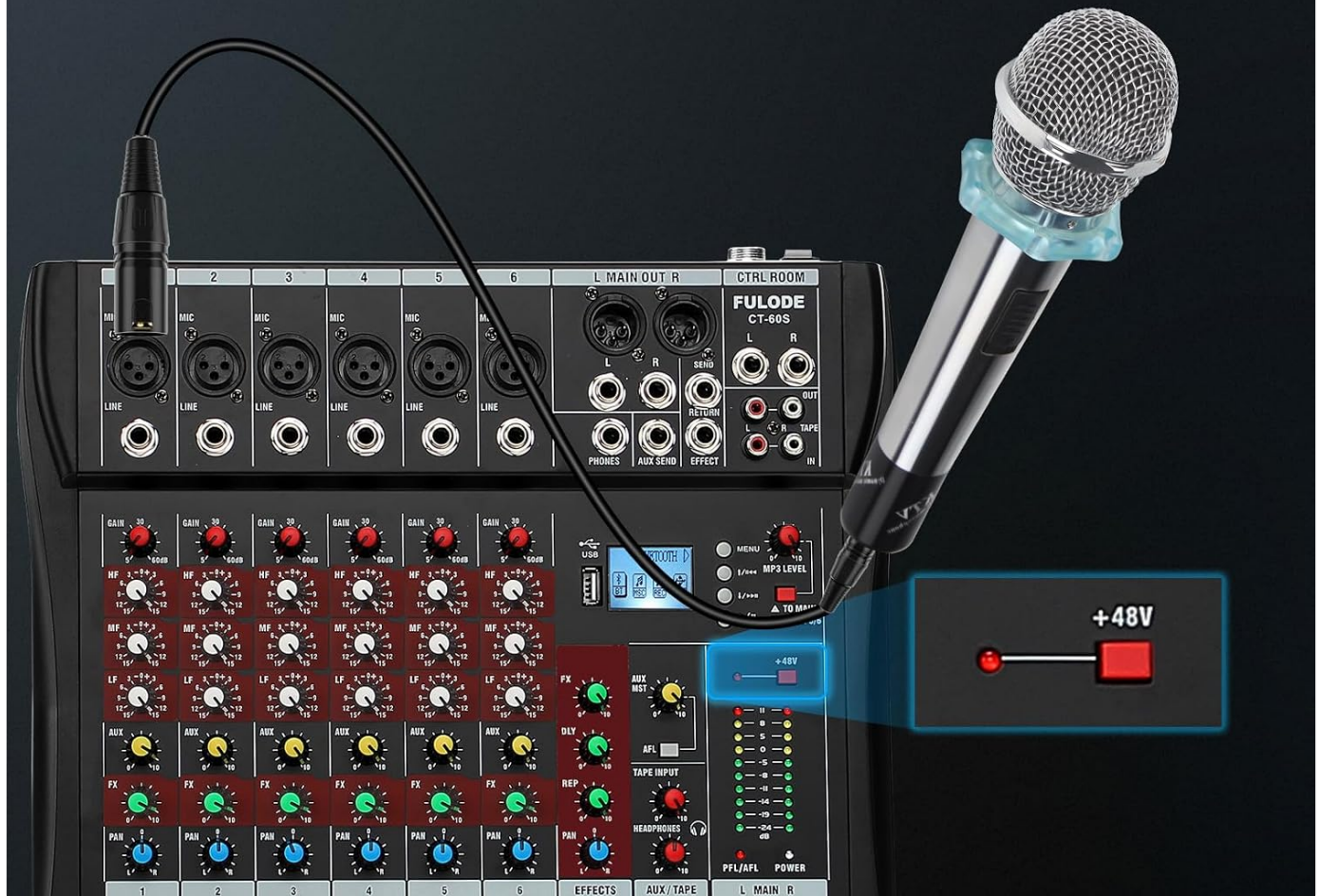
Figure 4.1: Connecting a Microphone with 48V Phantom Power
