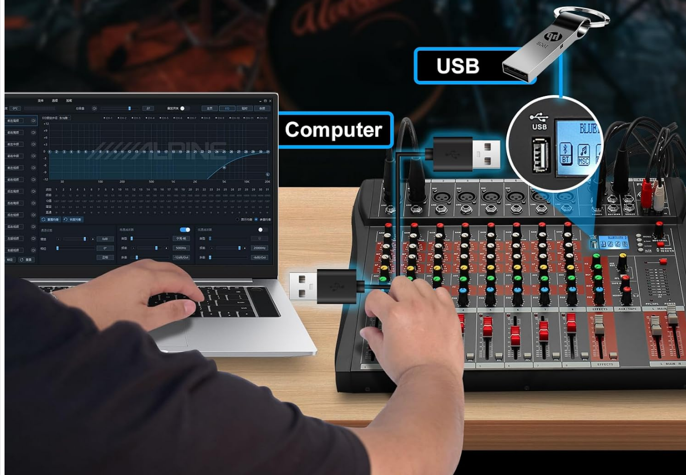
Figure 4.2: Connecting a USB device or computer to the mixer.
