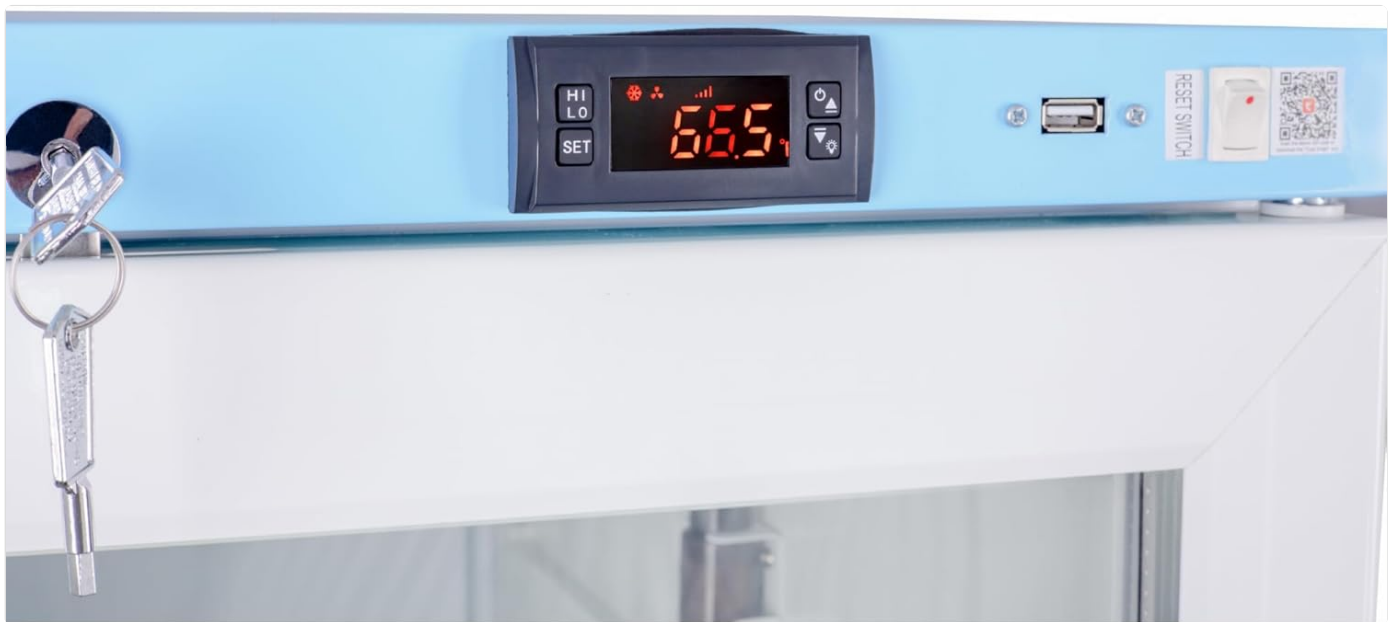
Figure 4: The electronic display panel provides control over various settings and shows the current temperature.
