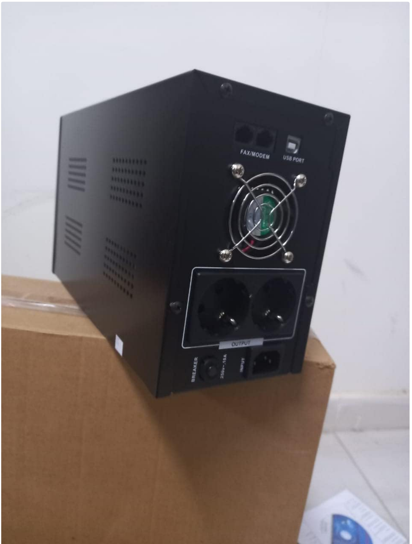
Figure 4.1: Rear view of the Dalton 2000VA UPS, highlighting the input power port, output sockets, and USB/Modem ports.
