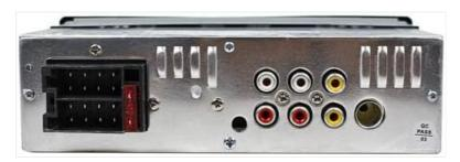
The rear view of the headunit shows the main power and speaker wiring harness connector on the left, along with multiple RCA output jacks for audio and video connections, and a fuse.
