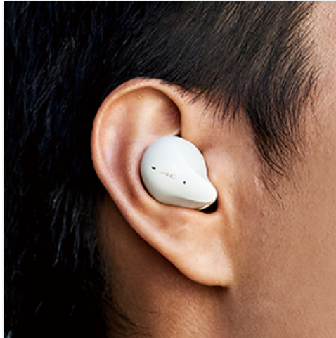
Image: Illustration of the press-and-hold gesture on an earbud to toggle between Noise Cancelling and Ambient Sound modes.
