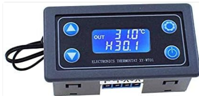
Figure 1: Front view of the XY-WT01 Digital Temperature Controller with its LCD display active.
