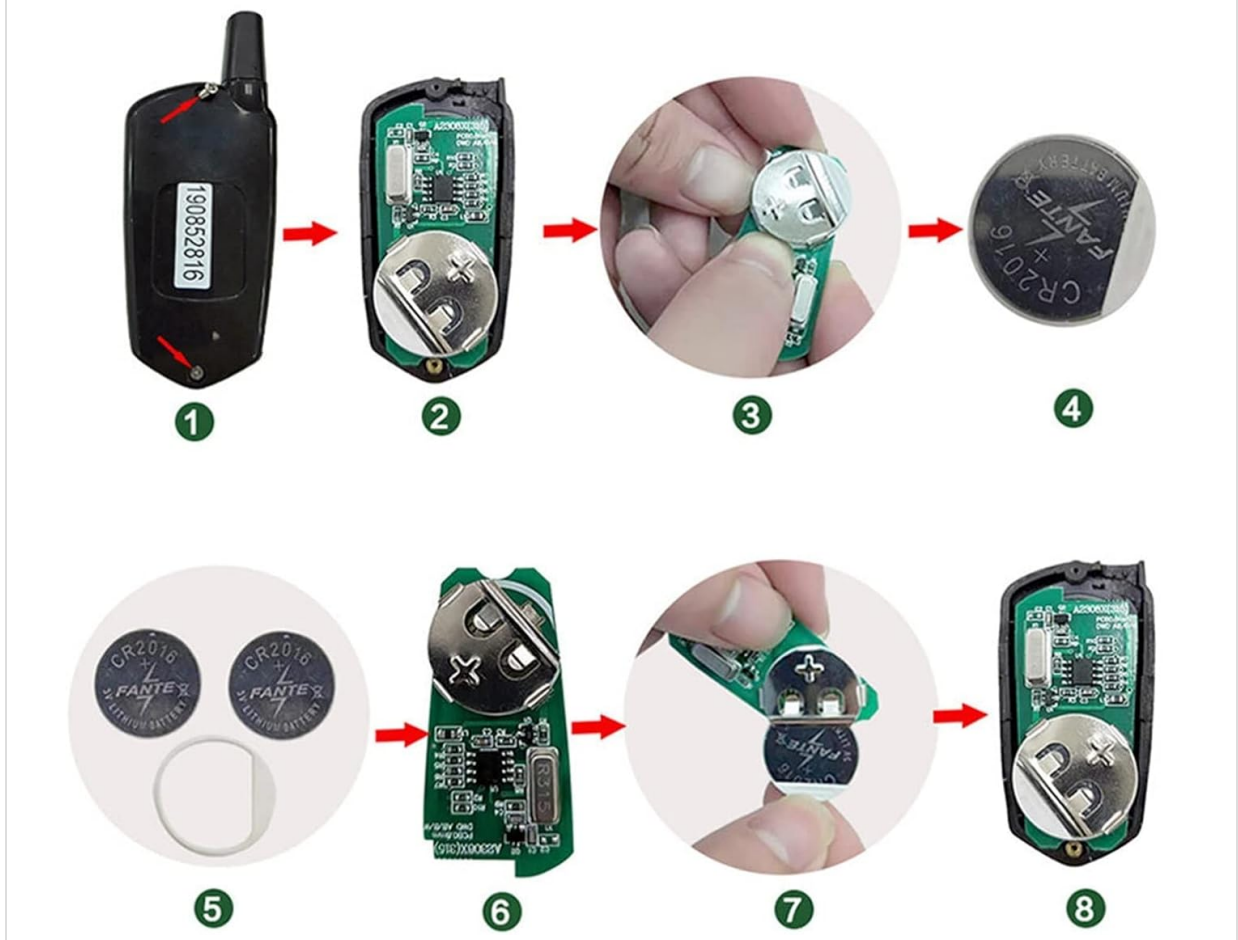
Image: A visual guide demonstrating the process of opening the remote control, inserting a CR2016 battery, and reassembling the unit.
