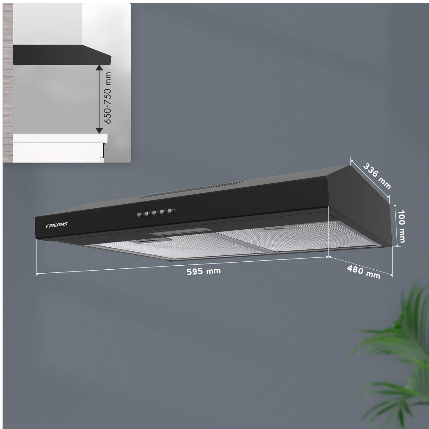
Image: Detailed dimensions of the extractor hood and the recommended mounting height range above a cooking hob.
