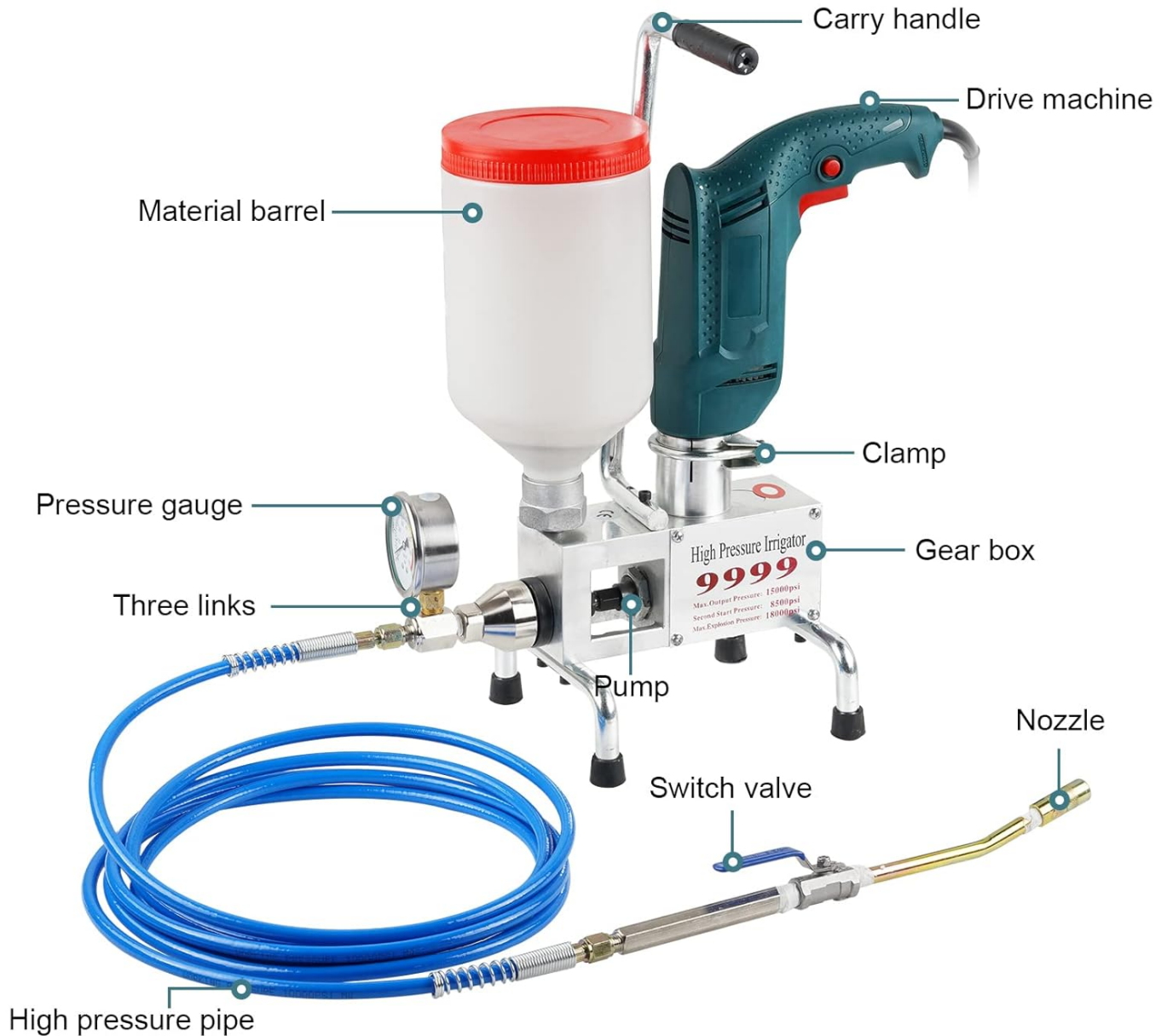
Figure 3.1: Labeled diagram of the grouting machine components, including the Carry handle, Drive machine, Material barrel, Pressure gauge, Three links, Pump, Switch valve, Nozzle, High pressure pipe, Clamp, and Gear box.
