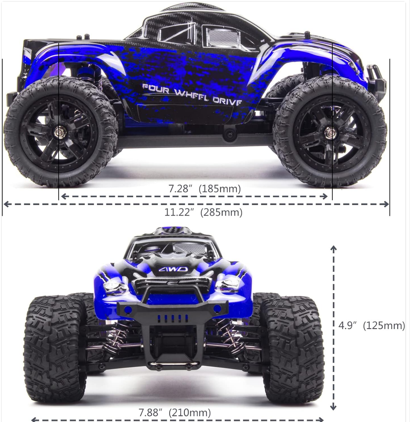
Figure 5: Visual representation of the RC truck's dimensions.
