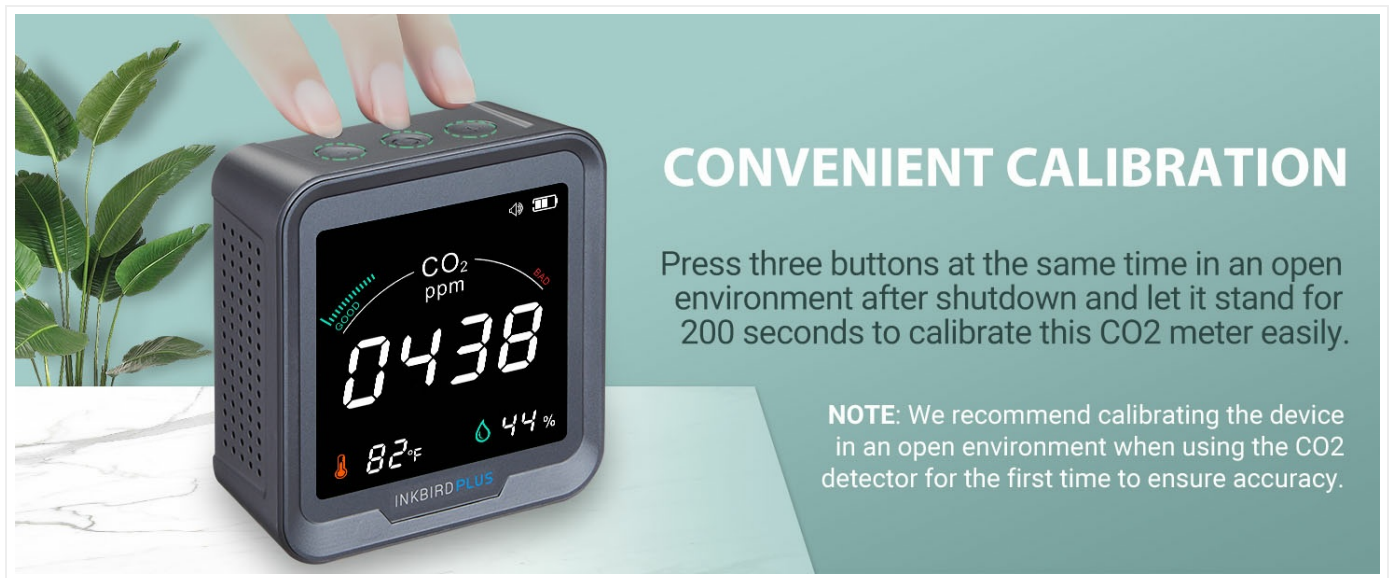
Figure 4: Illustration of pressing three buttons for CO2 calibration.
