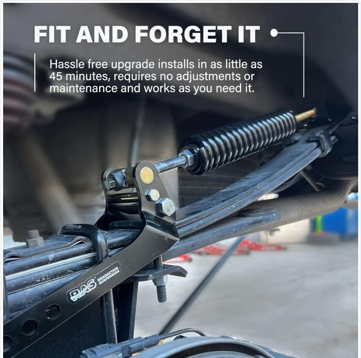
Image: An RAS unit securely mounted to a leaf spring, demonstrating the installation method.
