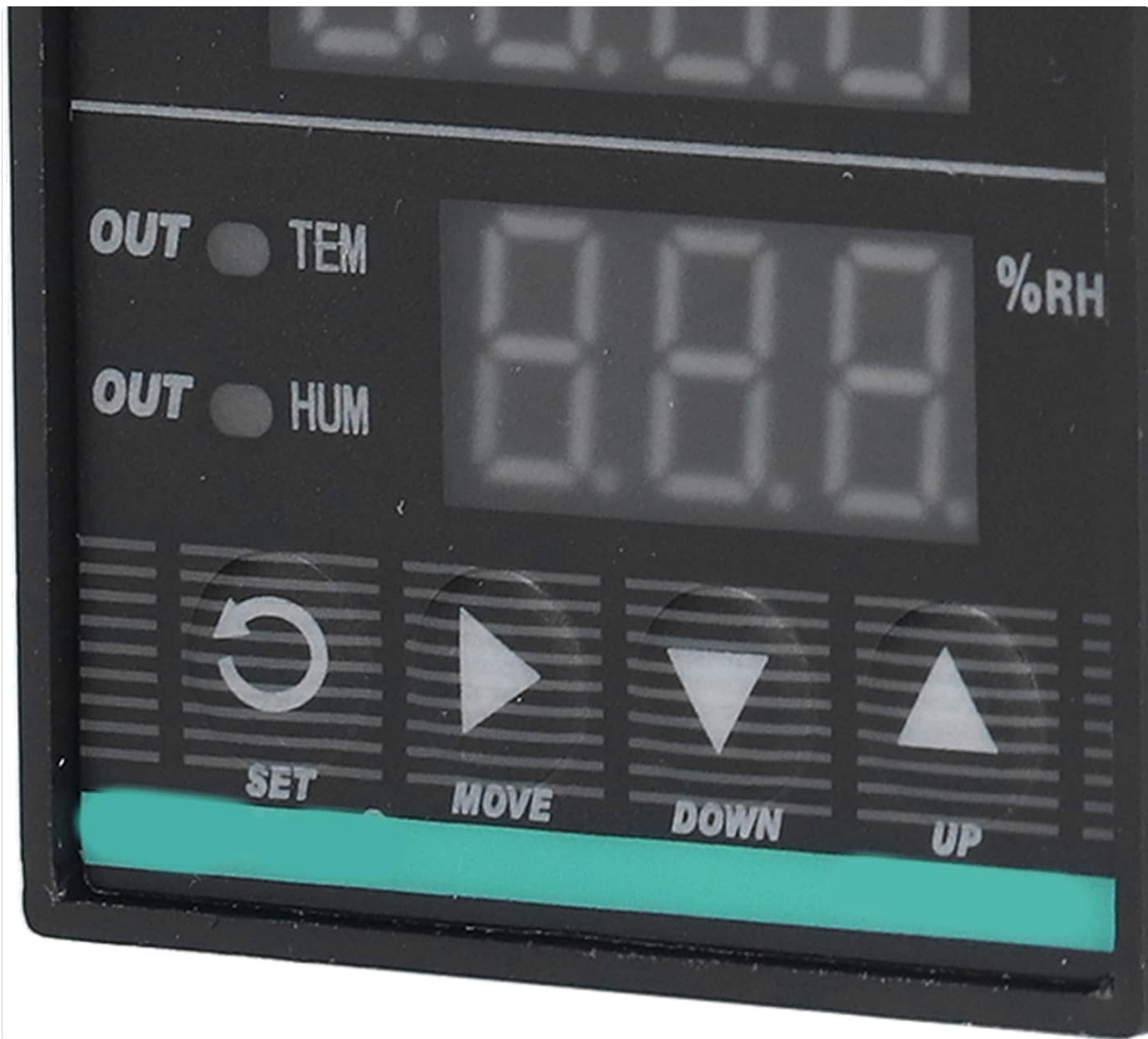
Figure 4: Close-up of display and buttons. Detailed view of the digital display showing temperature and humidity, with 'SET', 'MOVE', 'DOWN', and 'UP' buttons for parameter adjustment.
