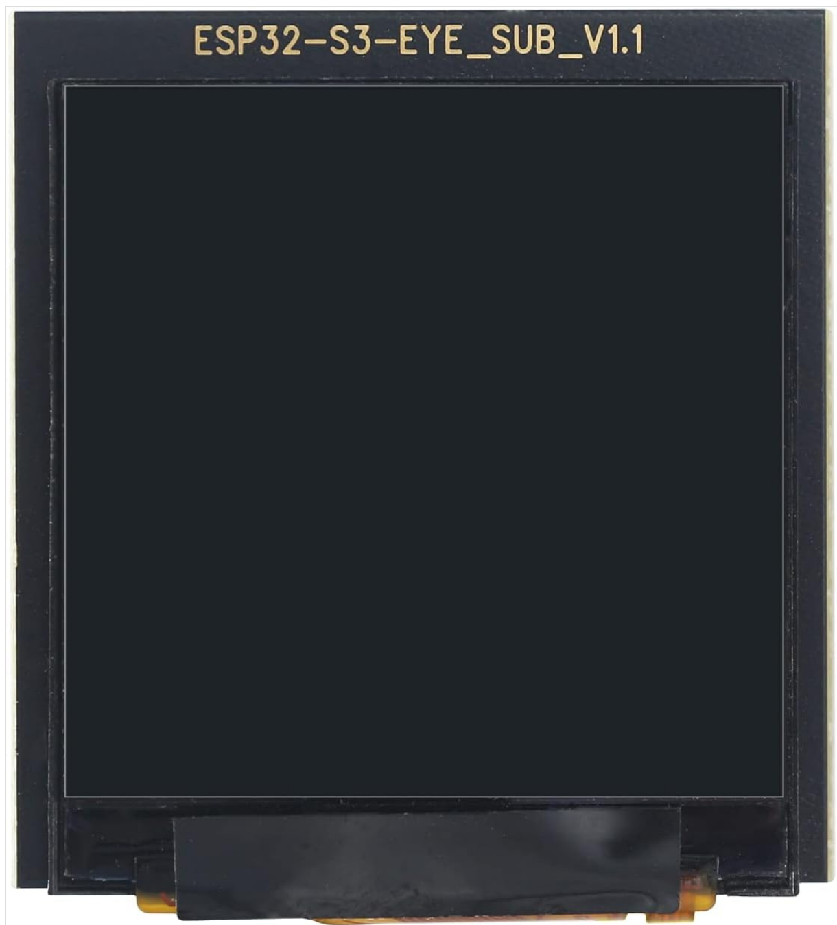
Figure 3.4: LCD Display Module. This image focuses on the 1.3-inch LCD display module, labeled ESP32-S3-EYE_SUB_V1.1. It shows the screen area and the flexible flat cable (FFC) connector at the bottom, which interfaces with the main board.
