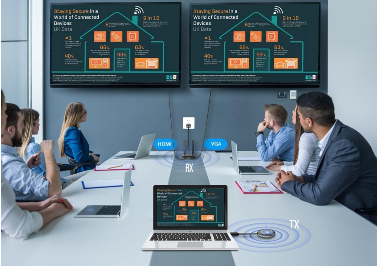
Image: Dual screen setup using HDMI and VGA outputs from the Receiver.
