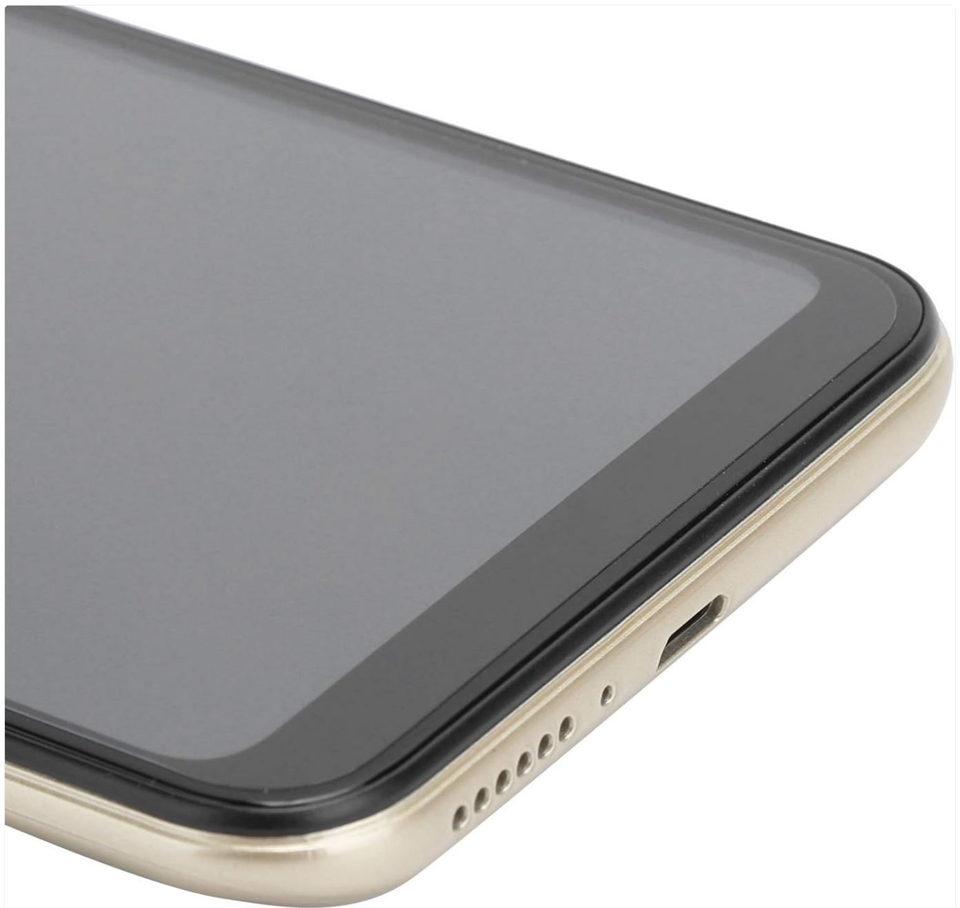
Figure 3.2: Detailed view of the smartphone's bottom edge, showing the USB charging port and speaker grille.
