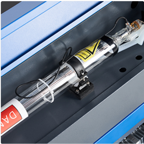
Figure 6: The CO2 laser tube, a critical component requiring proper cooling and care.
