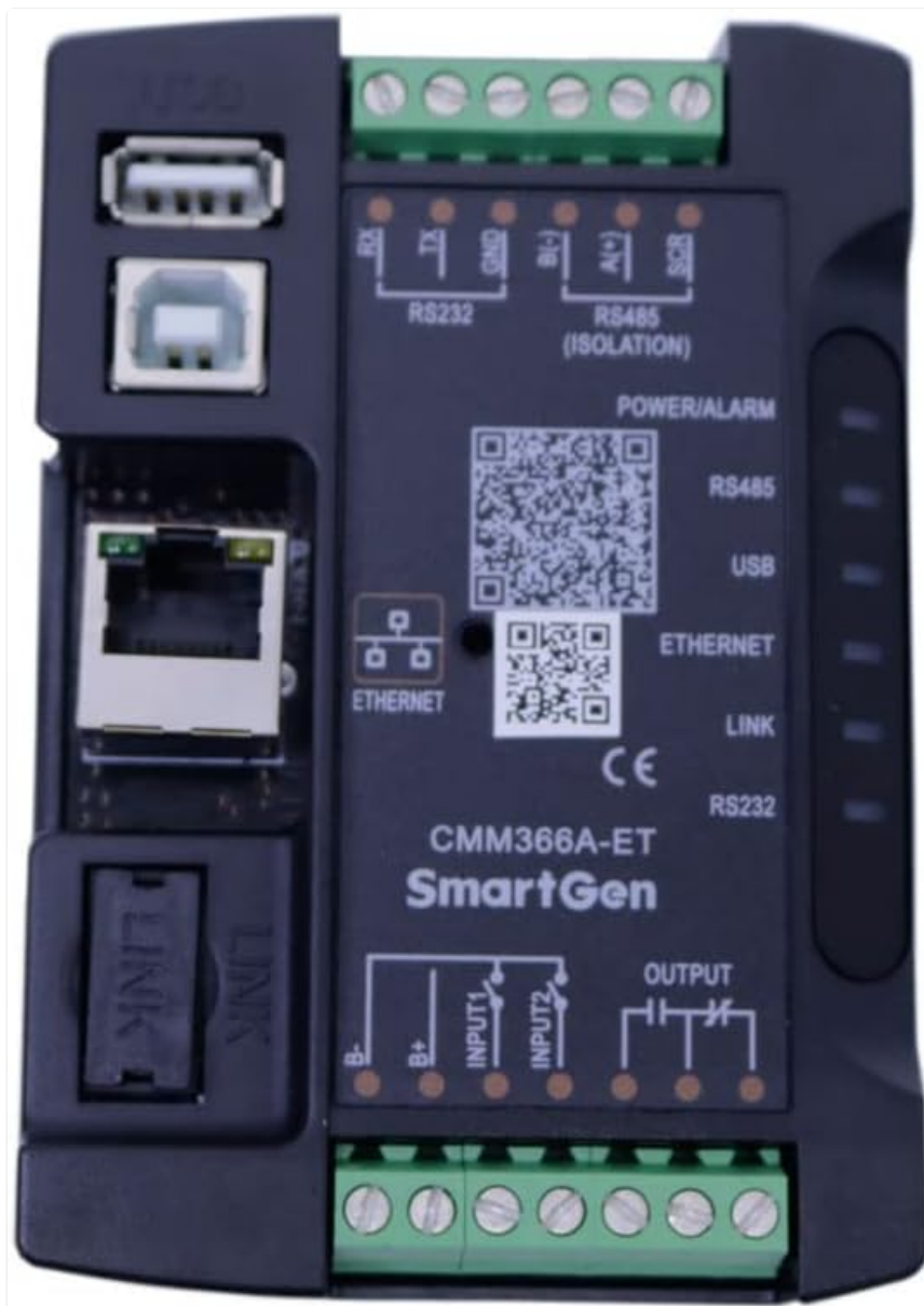
Figure 3.1: Front view of the CMM366A-ET module, highlighting USB, Ethernet, Link, RS232, RS485, and output terminals.
