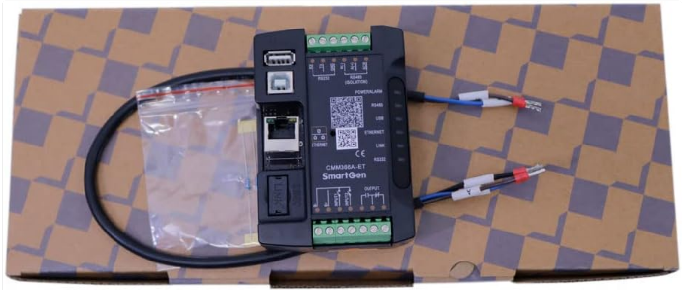
Figure 2.1: Smartgen CMM366A-ET module, connection cables, and instruction manual as packaged.
