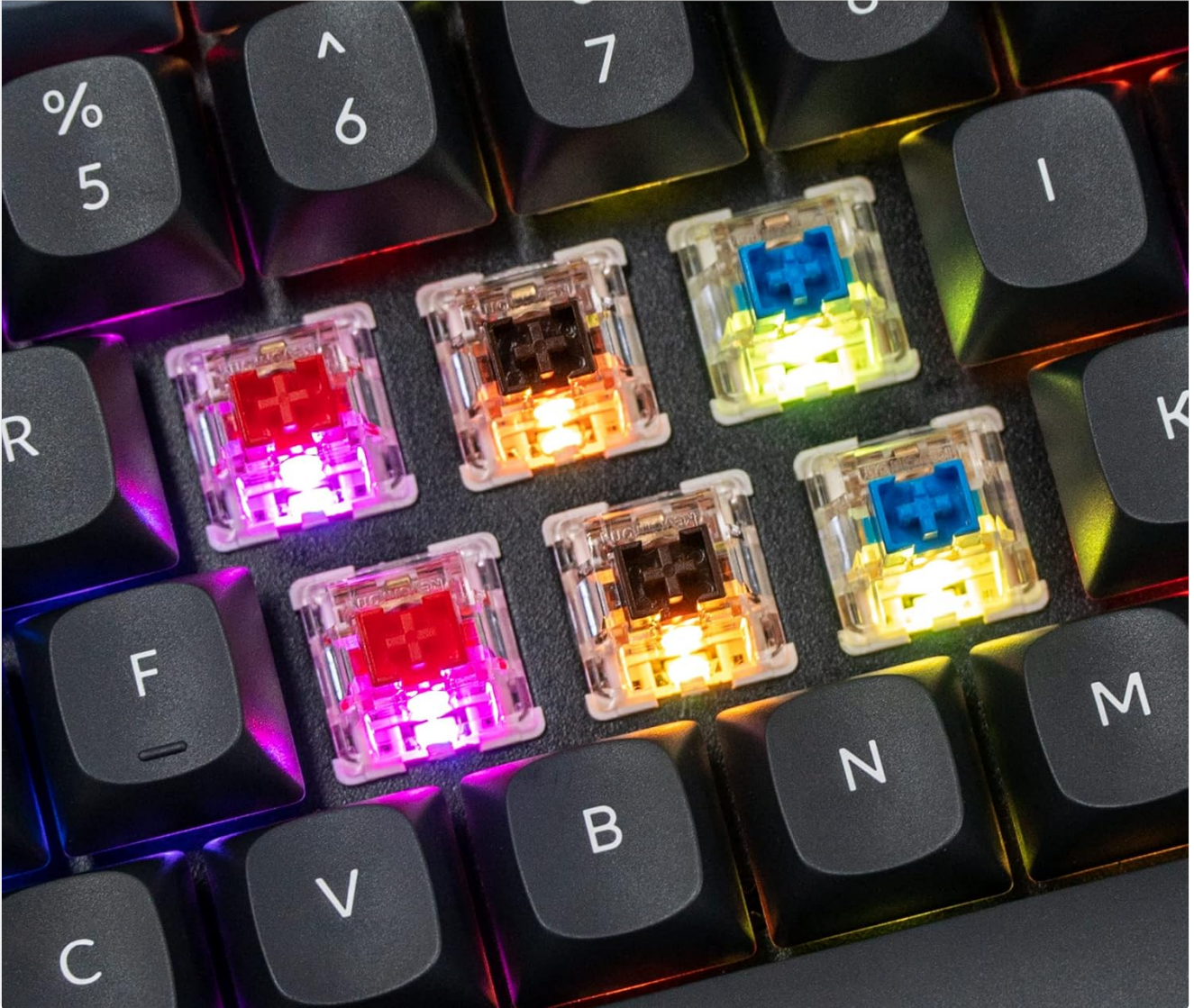
Image 4.3: Detail of the south-facing RGB lights illuminating the switches and keycaps from below.
