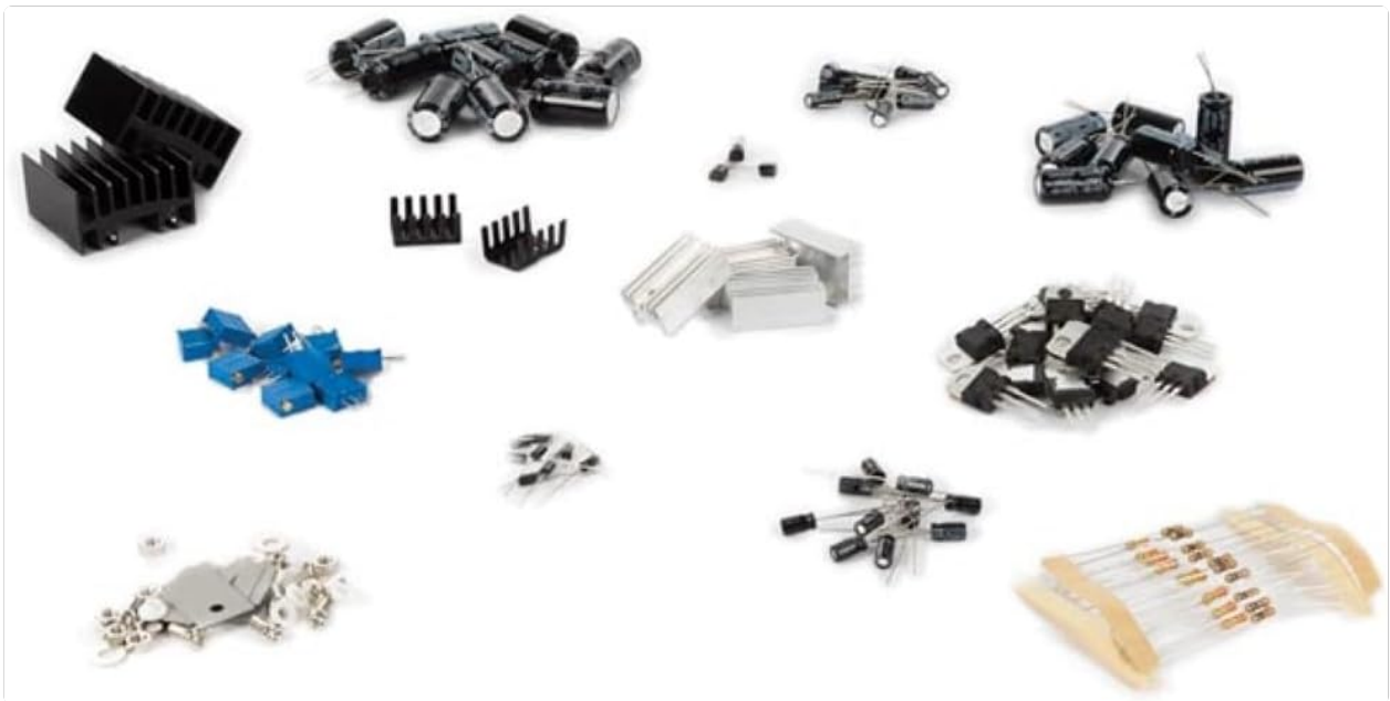
Image 2.2: A selection of components from the kit, including voltage regulators, capacitors, resistors, diodes, and heatsinks, laid out for inspection.
