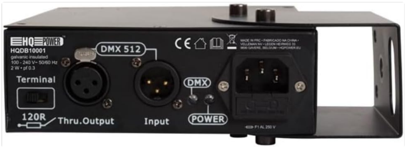
Image 3: Rear Panel - Power and DMX Input/Thru. This image shows the rear panel of the DMX splitter, including the AC power input, a 3-pin XLR DMX input, a 3-pin XLR DMX Thru output, and a 120R Terminal switch.
