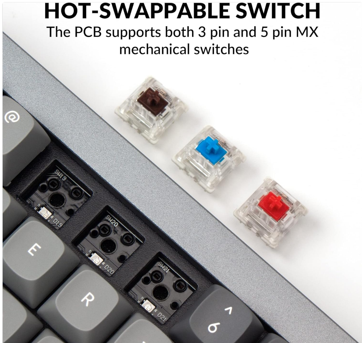
Image 4.2: Close-up view of the Keychron Q7's hot-swappable switch sockets with various Gateron switches.
