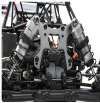
Image: A detailed view of the vehicle's shock absorbers and suspension components.
