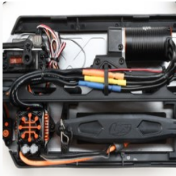
Image: Internal chassis view showing the layout of the ESC, motor, and wiring.
