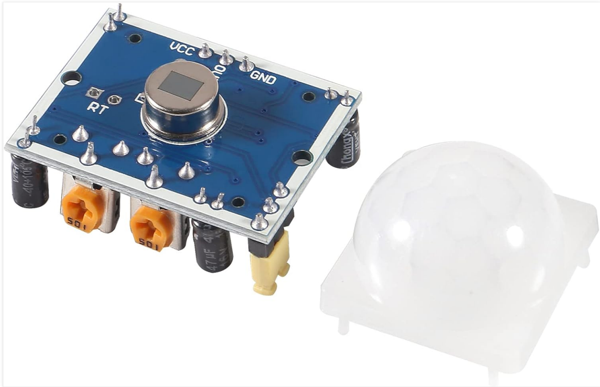
Figure 3: HC-SR501 module with lens removed, showing the pyroelectric sensor.
