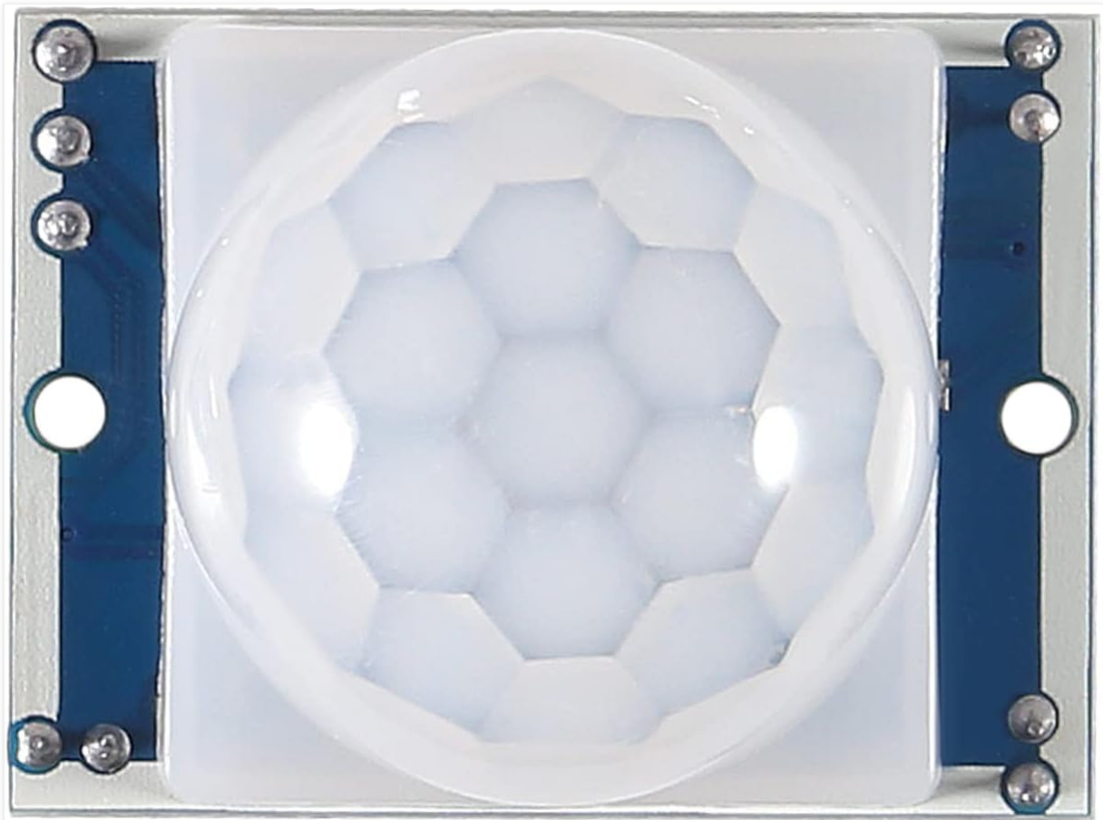
Figure 1: Top view of the HC-SR501 module showing the Fresnel lens.
