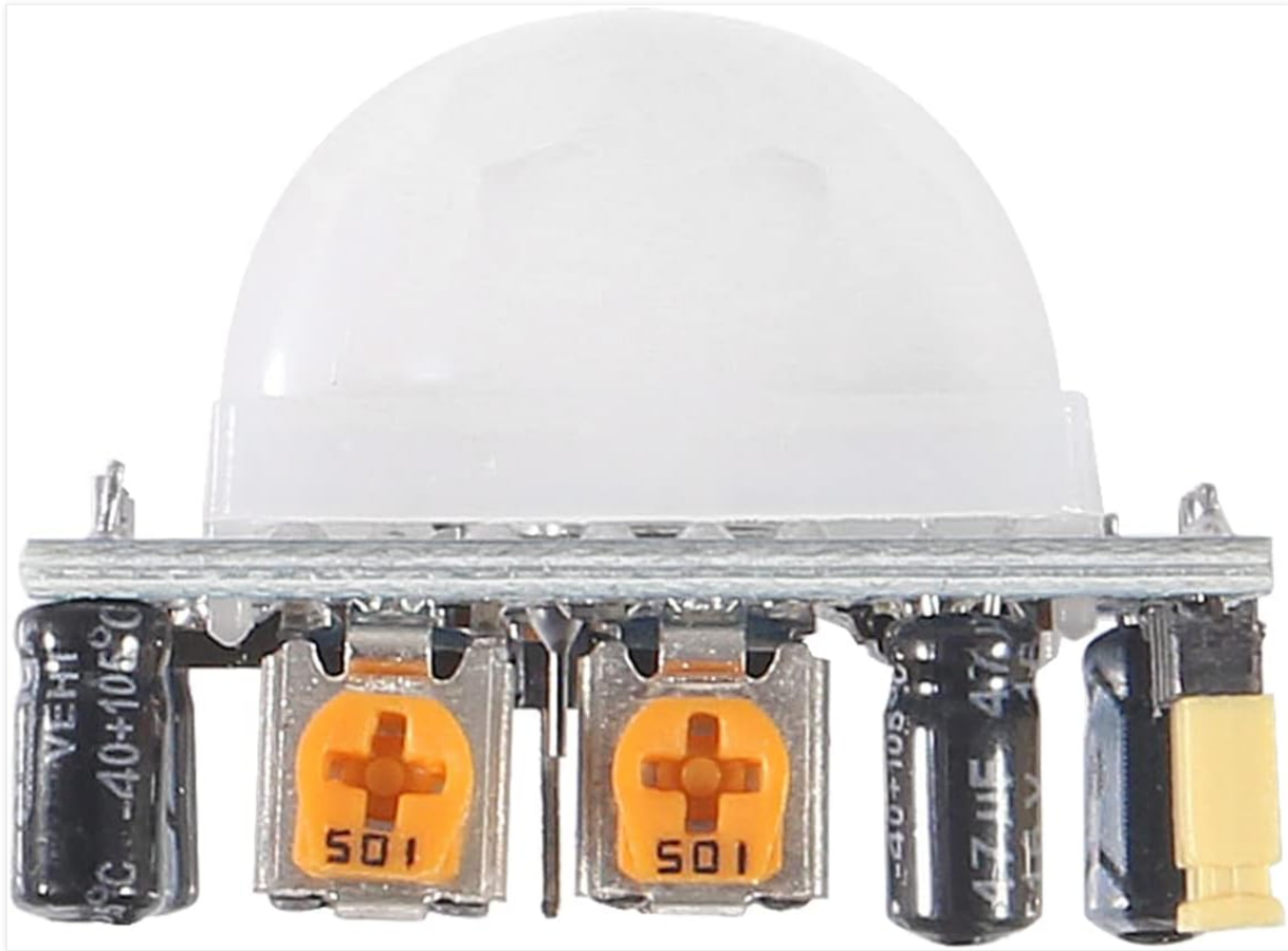
Figure 4: Potentiometers for adjusting delay time and sensitivity, and the trigger mode jumper.
