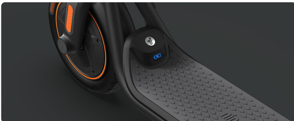
Figure 7: The integrated LED headlight for night riding.
