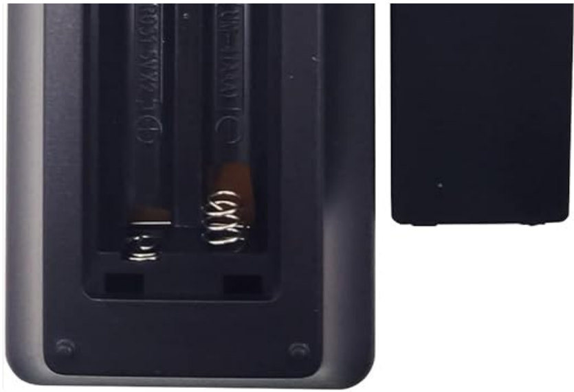
Figure 2: Back view of the remote control showing the open battery compartment and proper battery orientation.
