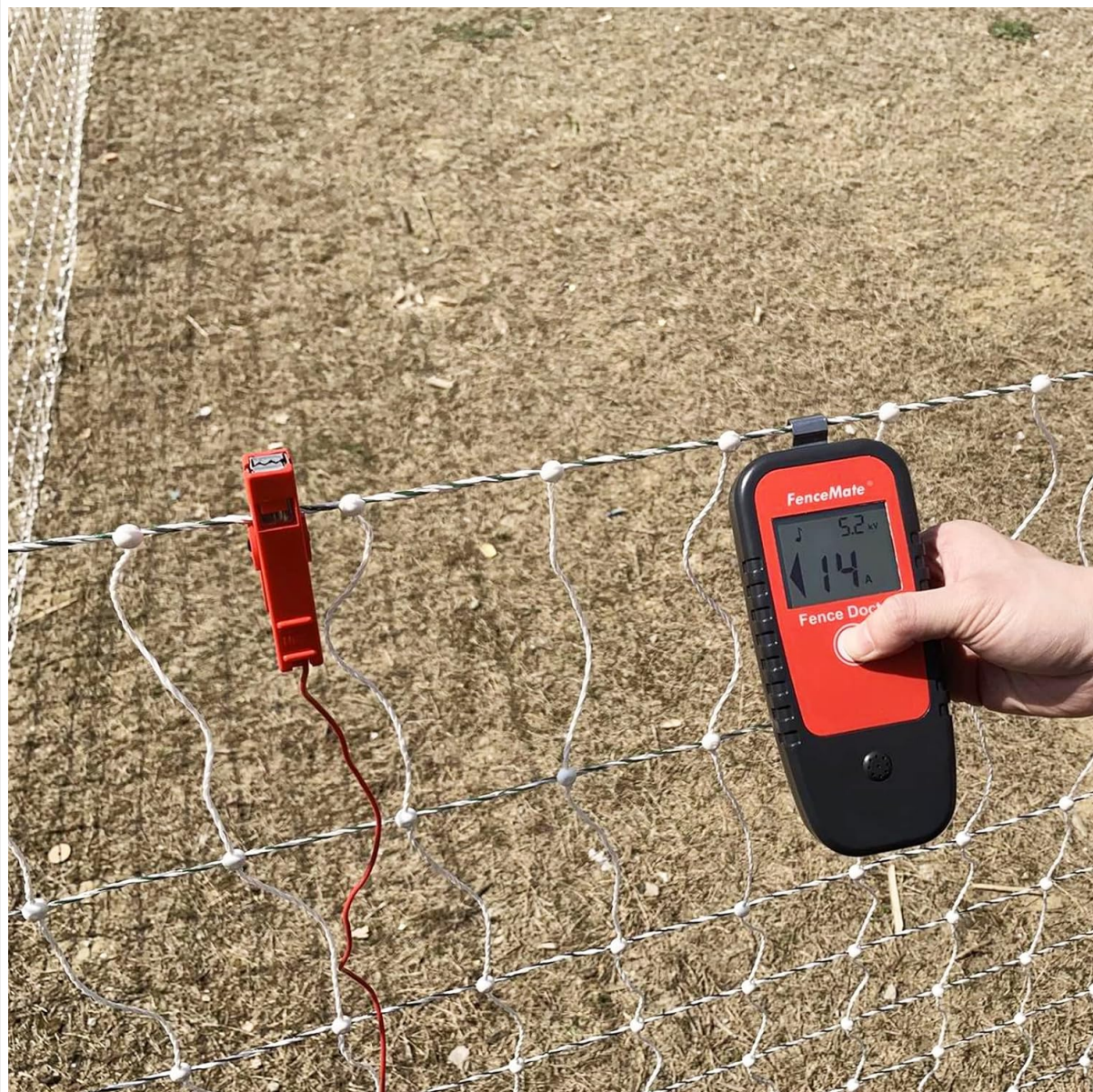
Image 3: The FenceMate Digital Fence Tester FT5502 actively measuring an electric fence. The display shows a voltage of 5.2 kV and a current of 1.14 A, indicating the fence is operational.
