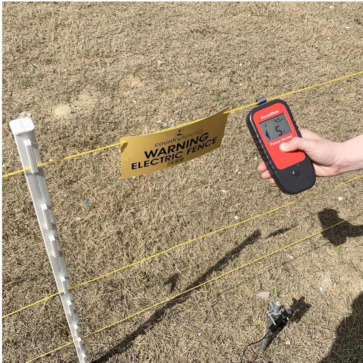
Image 4: The FenceMate Digital Fence Tester FT5502 being used to measure another electric fence, showing a reading of 4.5 kV and 1.5 A. A 'Warning Electric Fence' sign is visible in the background.
