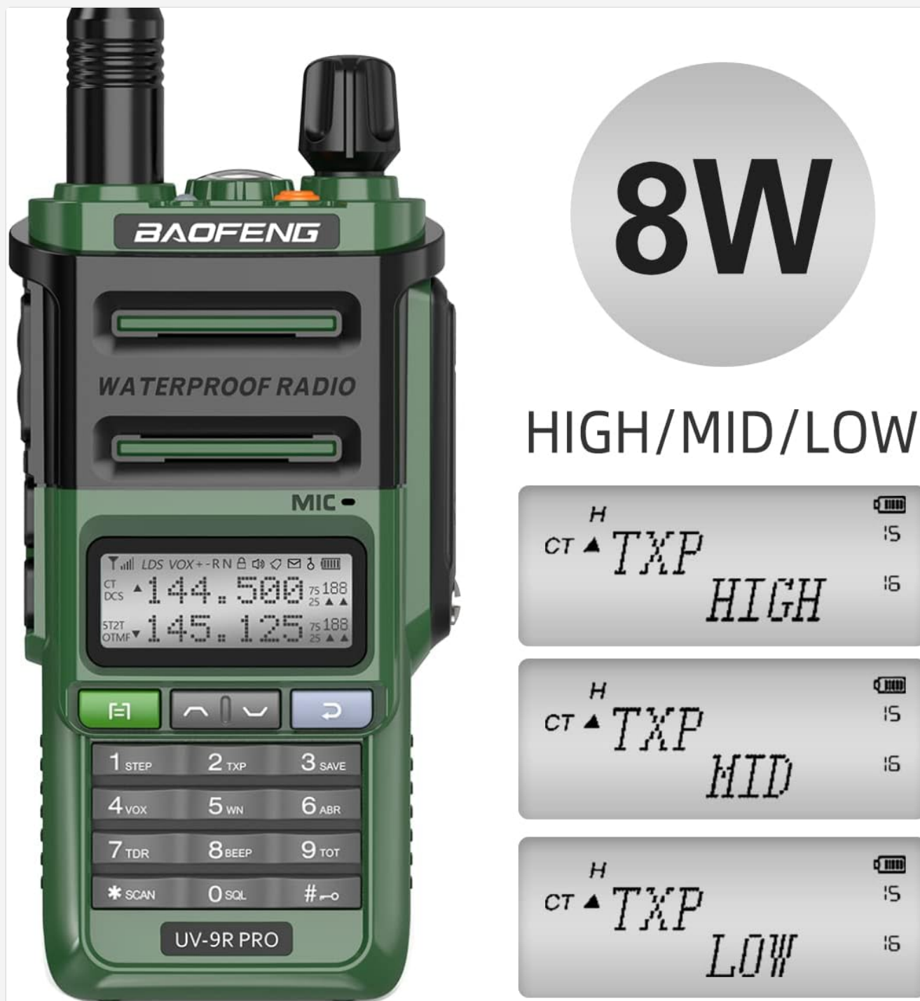
Image: The UV-9R Pro display showing options for High, Mid, and Low transmit power settings.
