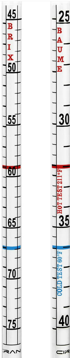
Image: Detailed view of the hydrometer's double Baume and BRIX scales, indicating hot and cold test lines.
