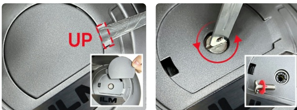
Figure 7: Details of the visor removal and installation mechanism, showing the 'UP' indicator and the retaining screw.
