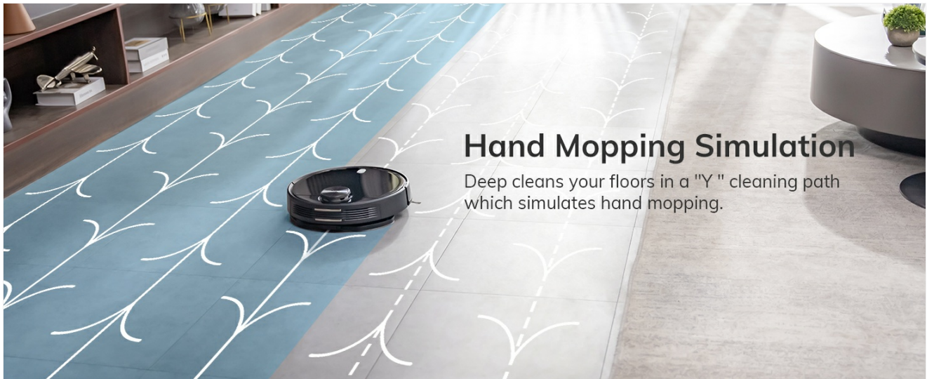
Figure 6.1: The robot performing its mopping function, illustrating the Y-shaped cleaning pattern for thorough floor coverage.
