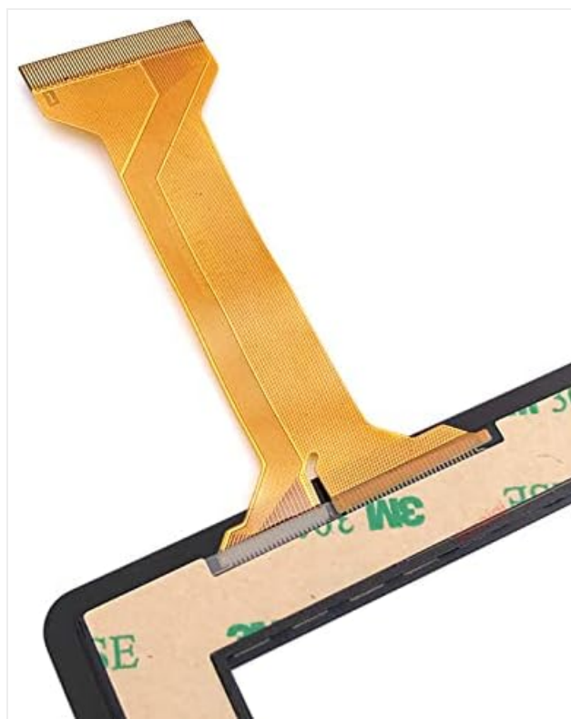
Figure 2: The digitizer with pre-applied adhesive and a close-up of the flex cable for connection.
