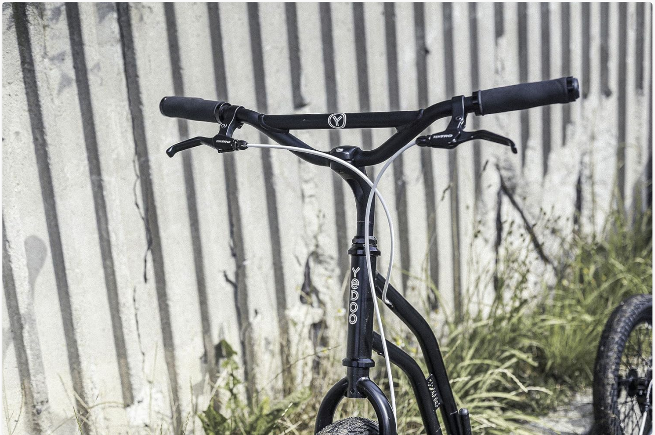
Figure 4: Detail of the handlebars, showing brake levers and ergonomic grips, important for regular inspection.
