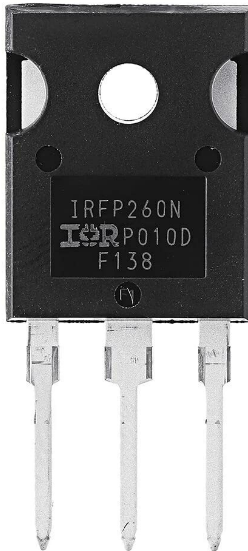
Figure 3.1: Front view of a single IRFP260N transistor, highlighting the model markings.
