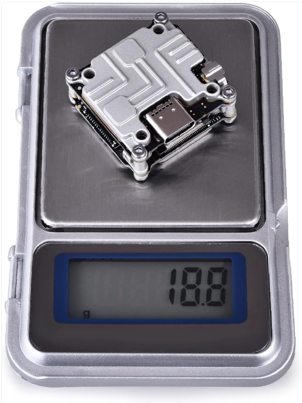
Figure 6: The module weighs approximately 18.8 grams.
