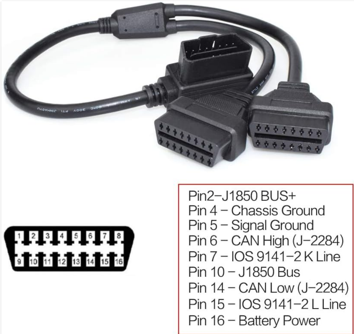
Figure 3: OBD2 Splitter Cable Pinout Diagram. This image shows the internal wiring connections for each pin on the OBD2 connector, detailing functions like J1850 BUS+, Chassis Ground, Signal Ground, CAN High, CAN Low, and Battery Power.
