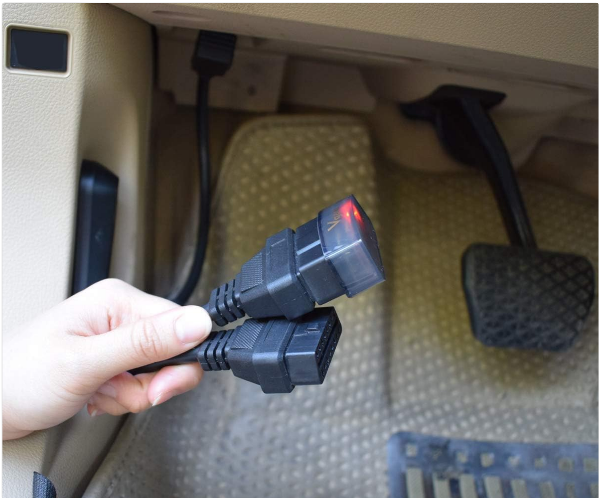
Figure 6: Vgate iCar Pro and Splitter Connected in Vehicle. This image shows the iCar Pro diagnostic tool connected to the OBD2 splitter, which is then plugged into the vehicle's OBD2 port, demonstrating a typical installation.
