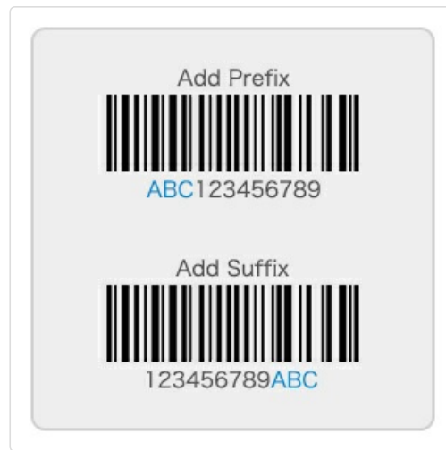
Image 6.2: Example of adding a prefix (ABC) or suffix (ABC) to a scanned barcode number.
