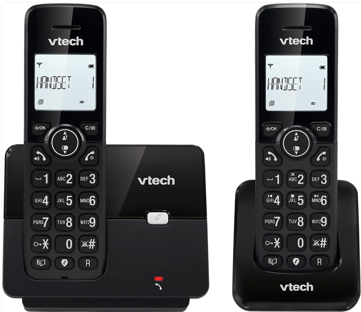
Figure 2.1: VTech CS2001 DECT Cordless Phone System. This image shows the VTech CS2001 DECT cordless phone system, which includes two handsets. One handset is docked in the main base unit, which connects to the telephone line, and the other handset is in its dedicated charging cradle. Both handsets feature a backlit display, large numeric keypad, and function buttons.
