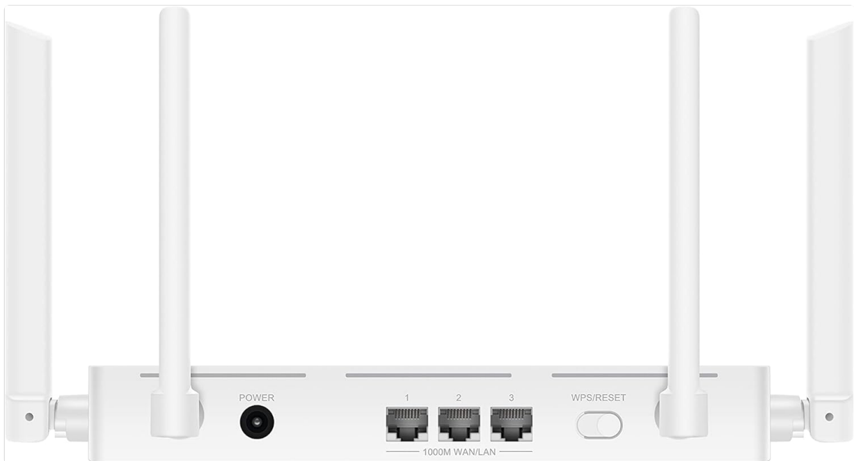
Image 3.1: Rear view of the HUAWEI WiFi AX2 Router, showing the power port, three LAN/WAN ports, and the WPS/Reset button.
