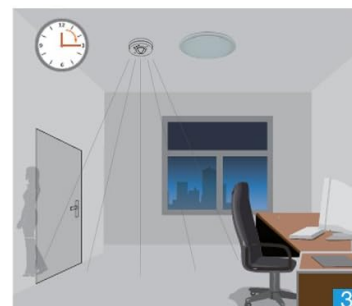
With insufficient natural light, the sensor switches OFF the light automatically when no more movement is detected.
