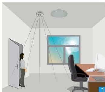
With sufficient natural light, the light does not switch on, even when movement is detected.
