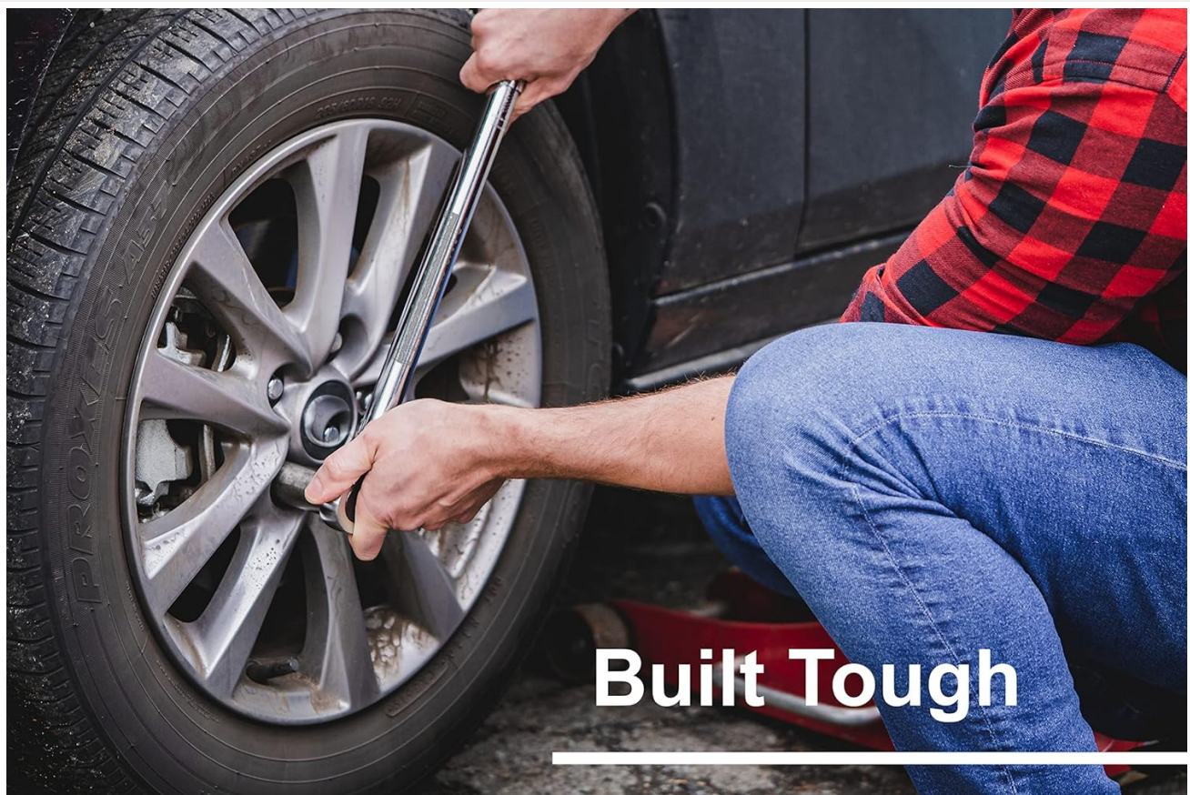
Figure 3: Proper application of the torque wrench for tightening fasteners, such as lug nuts.
