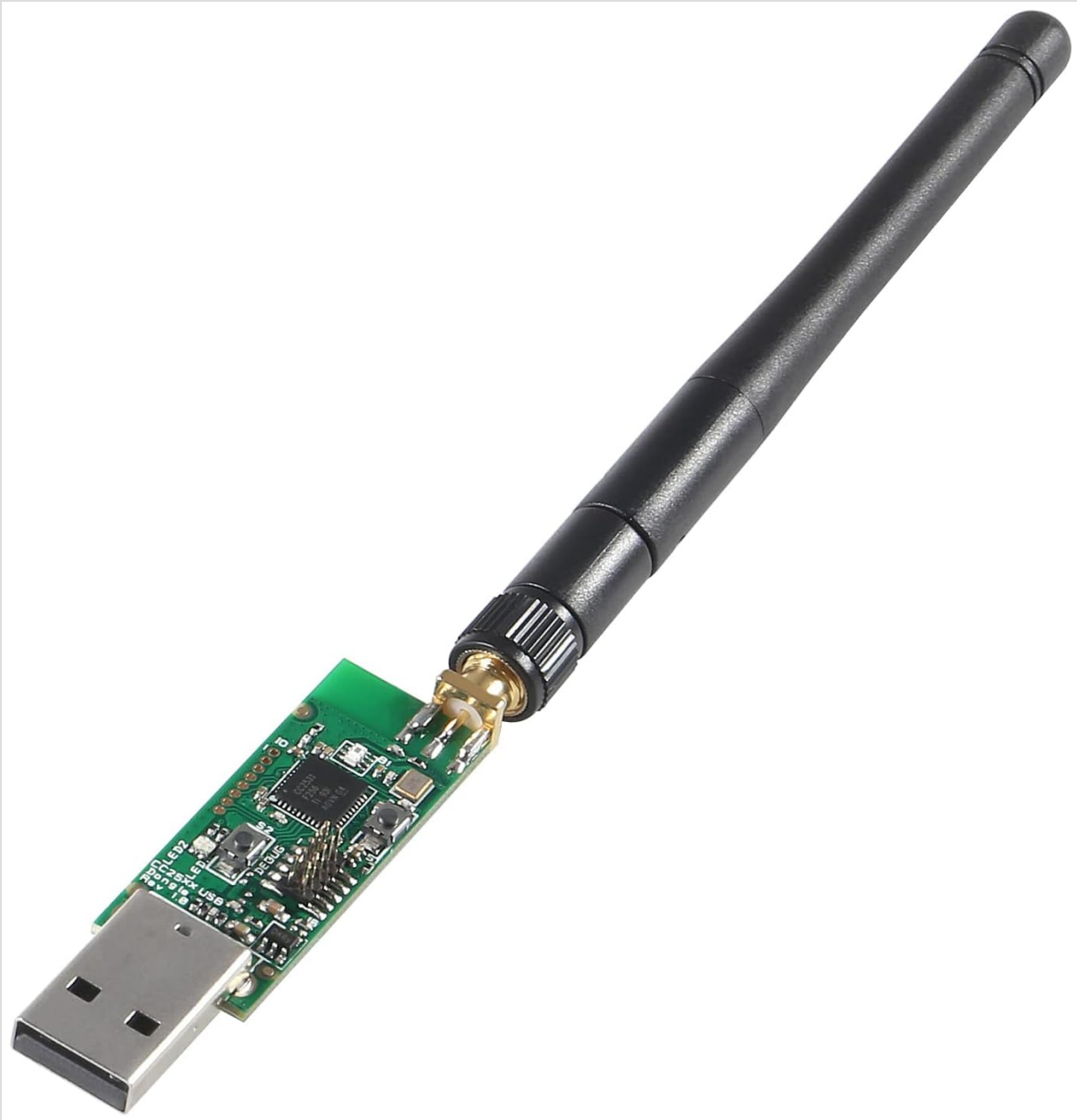
Figure 4: Top view of the CC2531 USB Dongle with its external antenna connected.
