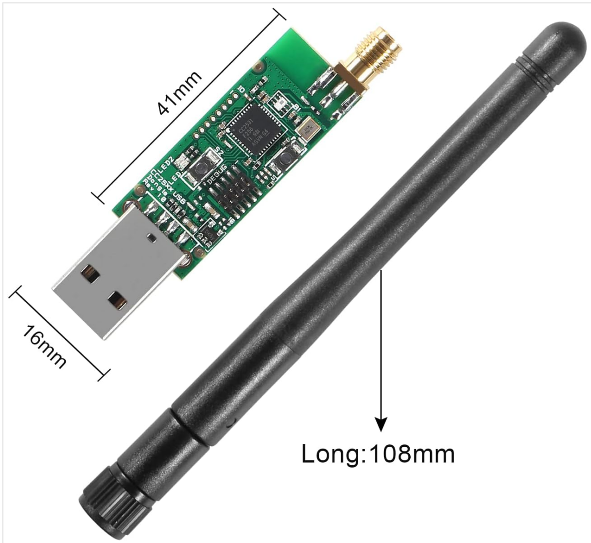
Figure 5: Dimensions of the CC2531 USB Dongle (41mm x 16mm) and the external antenna (108mm long).
