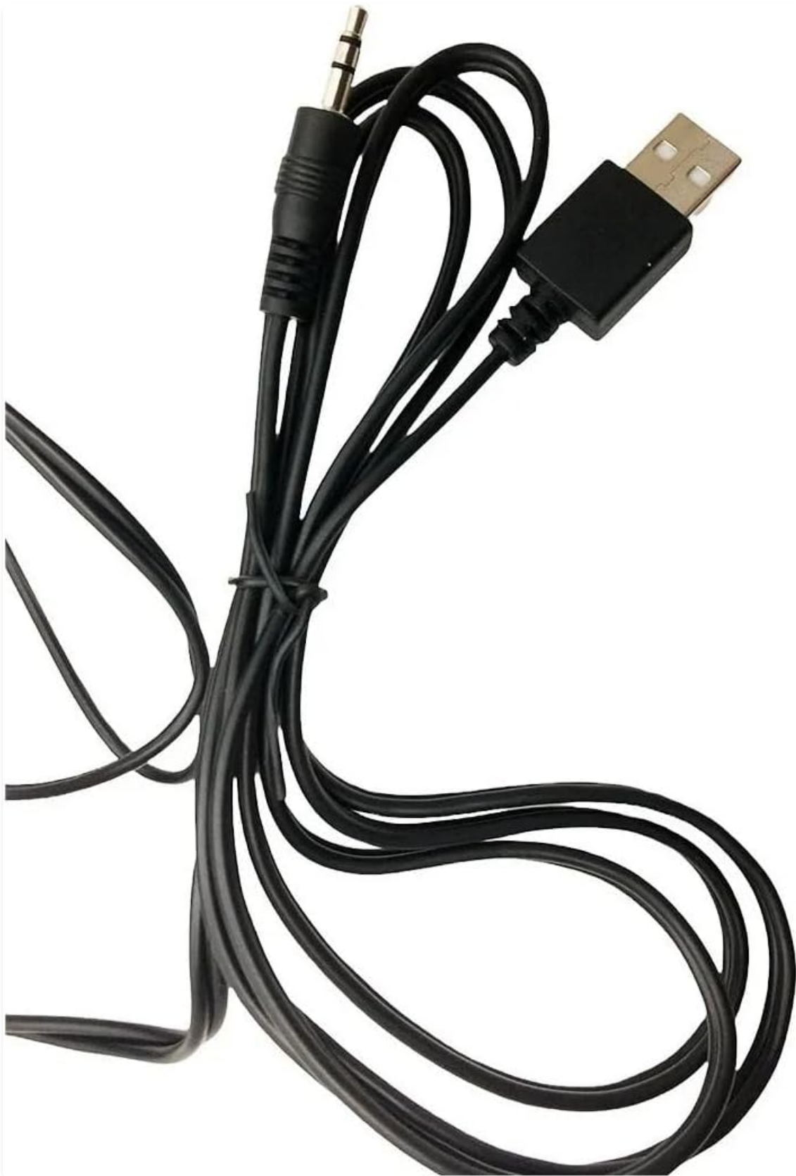
Figure 2: Integrated USB power and 3.5mm audio cables.
