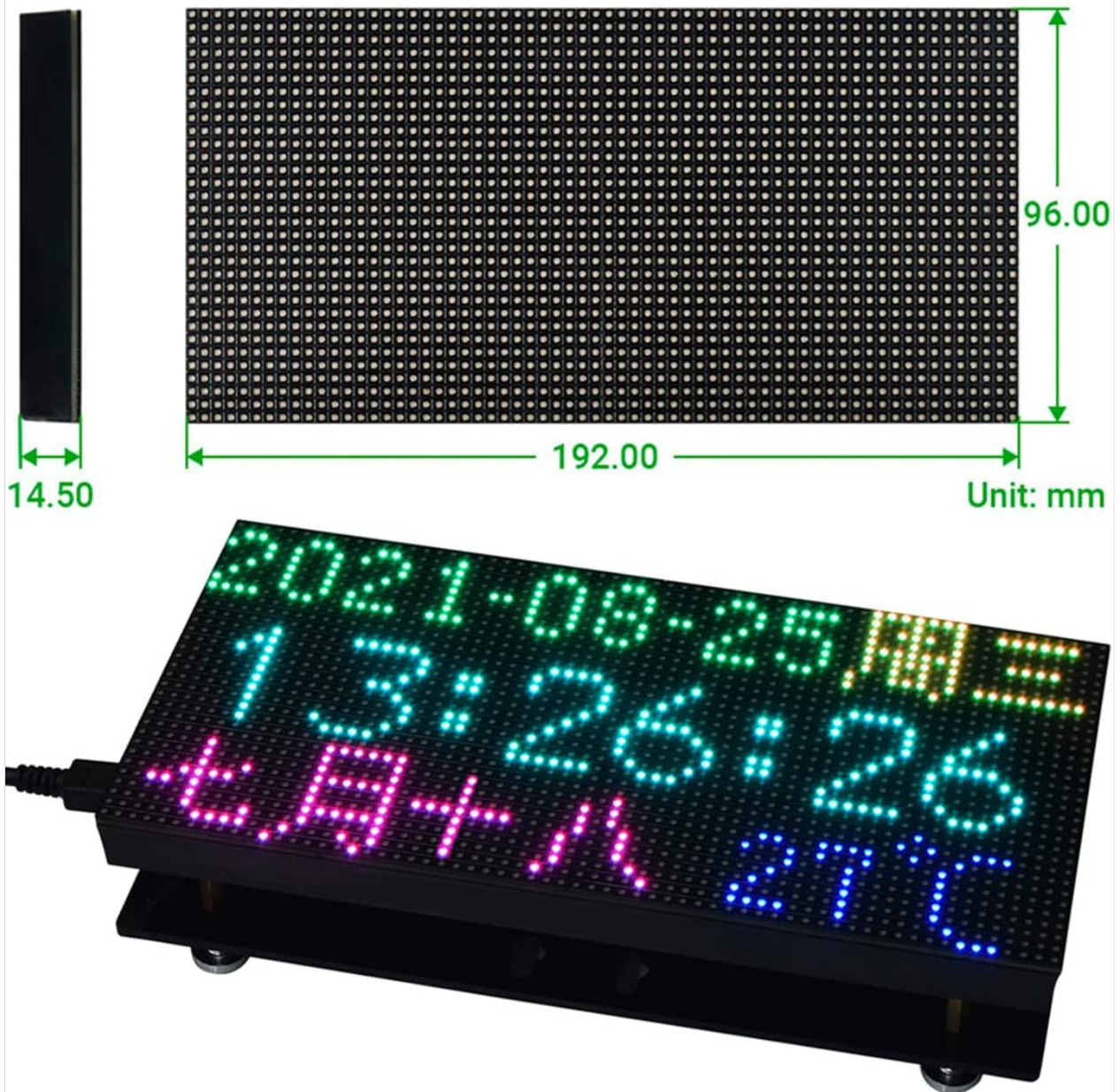
Figure 5: Physical dimensions of the LED Matrix Panel.
