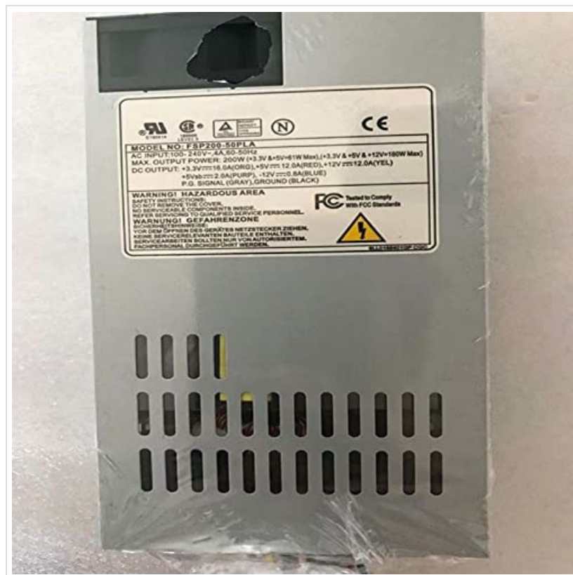
Figure 5: Detailed view of the power supply's specification label, showing model number, input/output voltages, and current ratings for different rails.
