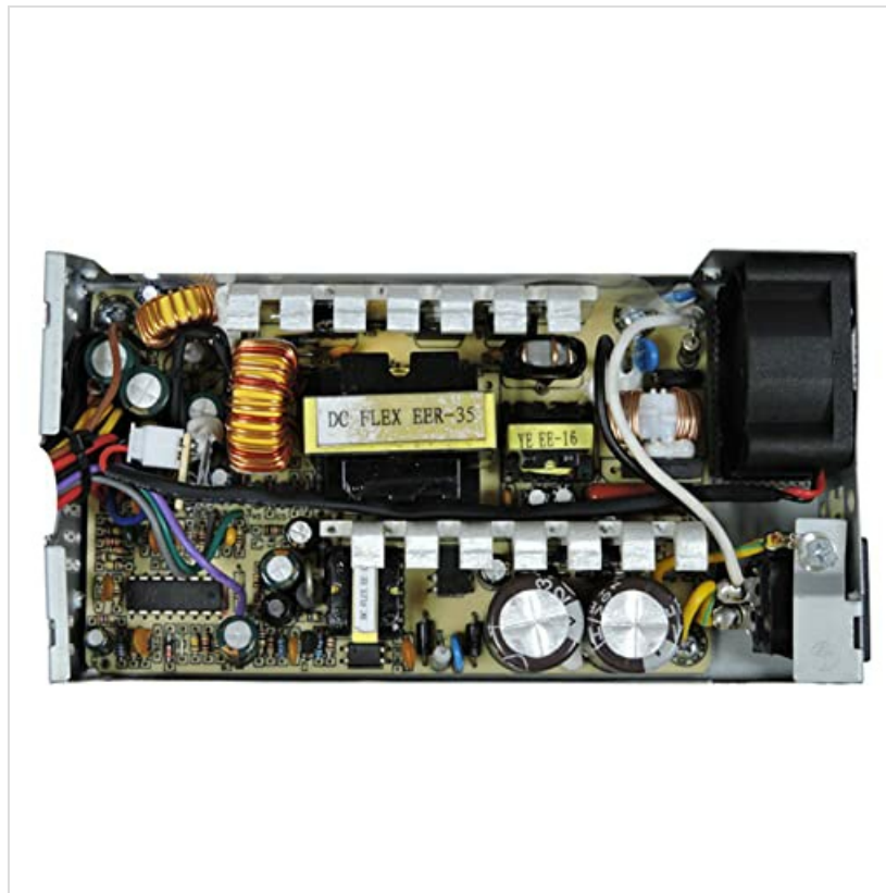
Figure 4: Internal view of the power supply unit, showing the circuit board, capacitors, coils, and other electronic components. This view is for informational purposes only; users should not open the PSU casing.
