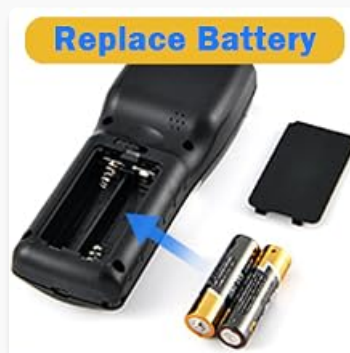
Figure 4: Battery replacement instructions for the scanner.
