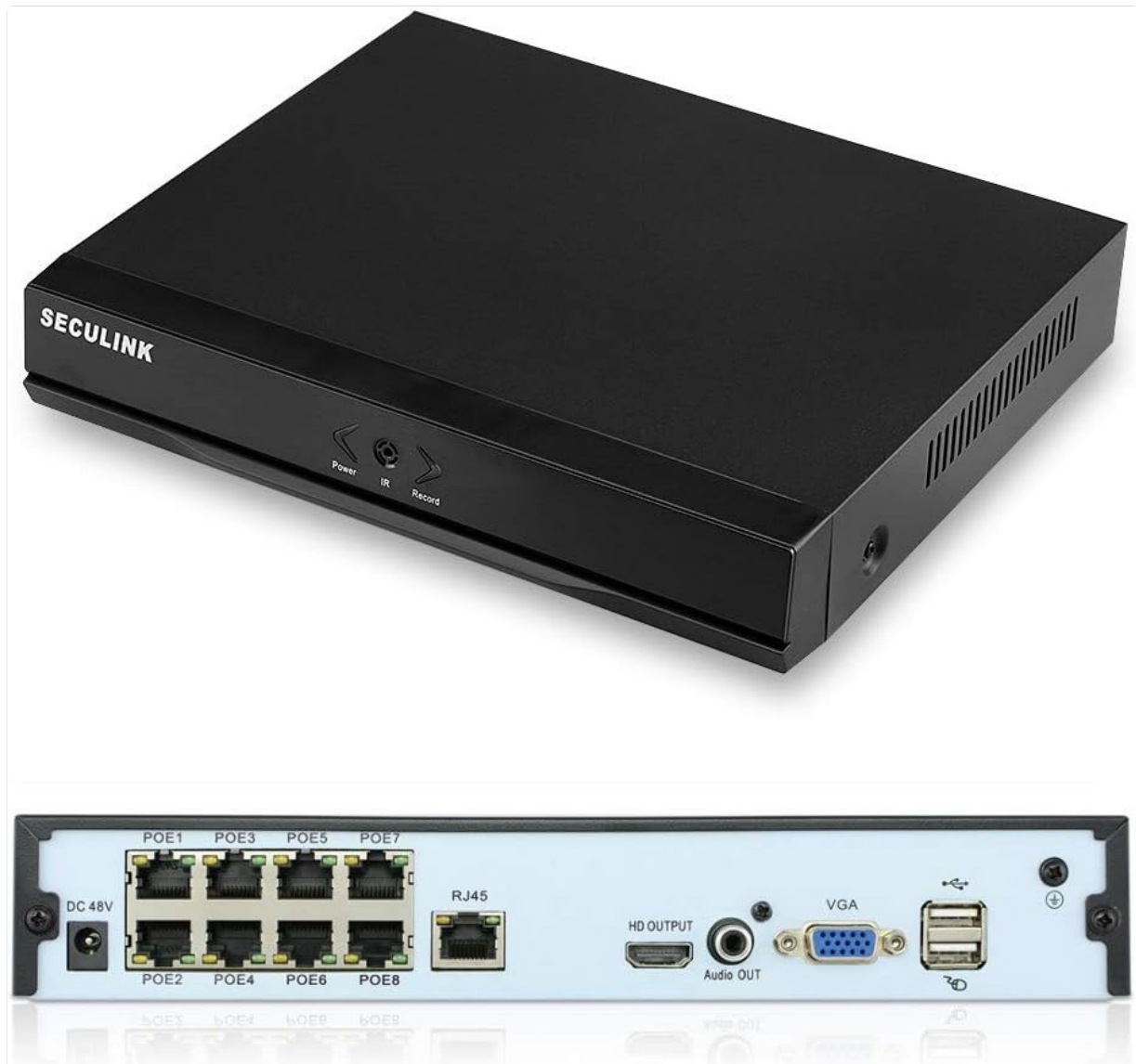
Figure 3.1: Top and Rear View of the NVR. The rear panel features 8 PoE ports for camera connections, an RJ45 uplink port, HDMI and VGA video outputs, an audio output, DC 48V power input, and USB ports for mouse and external storage.
