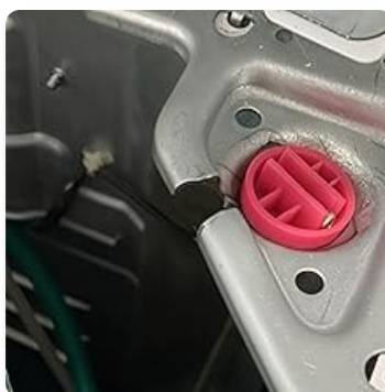
Image: A detailed shot showing the top red cap of a suspension rod being inserted into its designated slot on the washer tub, illustrating the final step of securing the rod.
