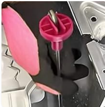
Image: A close-up view of a new suspension rod correctly installed into its mounting point within the washing machine's frame, demonstrating the secure fit of the damper assembly.
