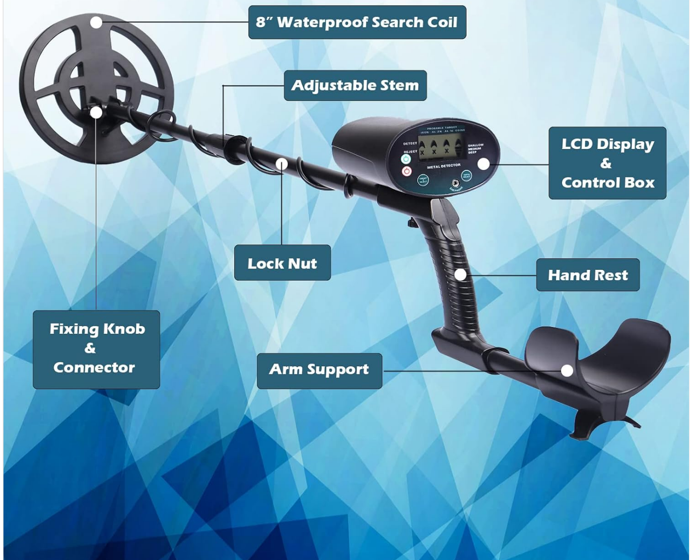
Image 2: Labeled components of the GT620G Metal Detector, including the 8" waterproof search coil, adjustable stem, LCD display & control box, hand rest, arm support, fixing knob & connector, and lock nut.
