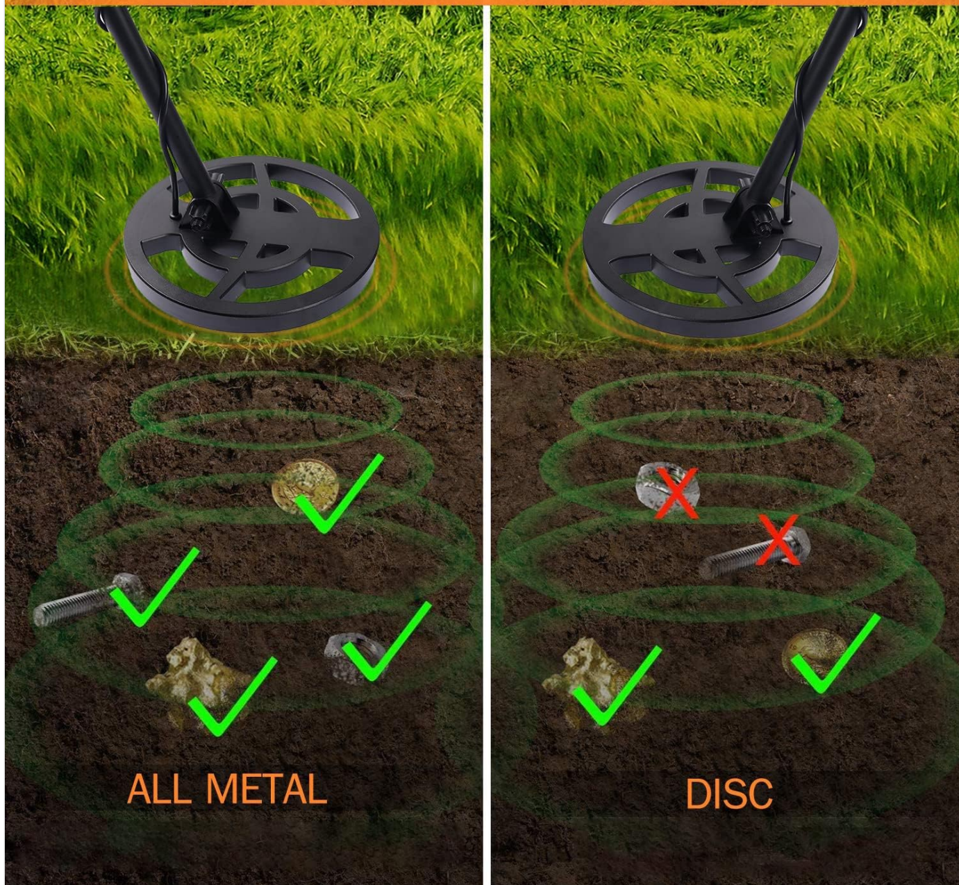
Image 5: Illustrates the difference between All Metal Mode (detects all metals) and DISC Mode (rejects specific metals like iron and screws).
