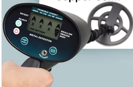
Image 4: Visual guide for activating All Metal Mode and DISC Mode. For All Metal Mode, adjust sensitivity via 'DEPTH SELECT'. For DISC Mode, use 'Target X Reject' to eliminate iron, and press again to reject copper coins.
